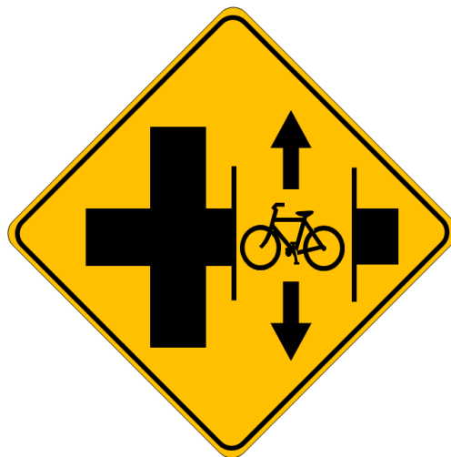
Figure 14-45 Example ADJACENT PATH Sign
